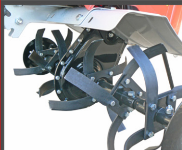
Carter in lamiera stampata con gusci avvitati Gear housing in press-formed plate sections secured by bolts
