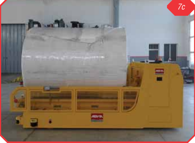
Application in paper field for mother reels. Handling solution for reels up to 10 tons
