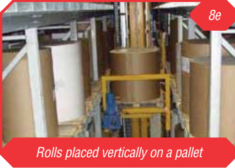
Rolls placed vertically on a pallet
