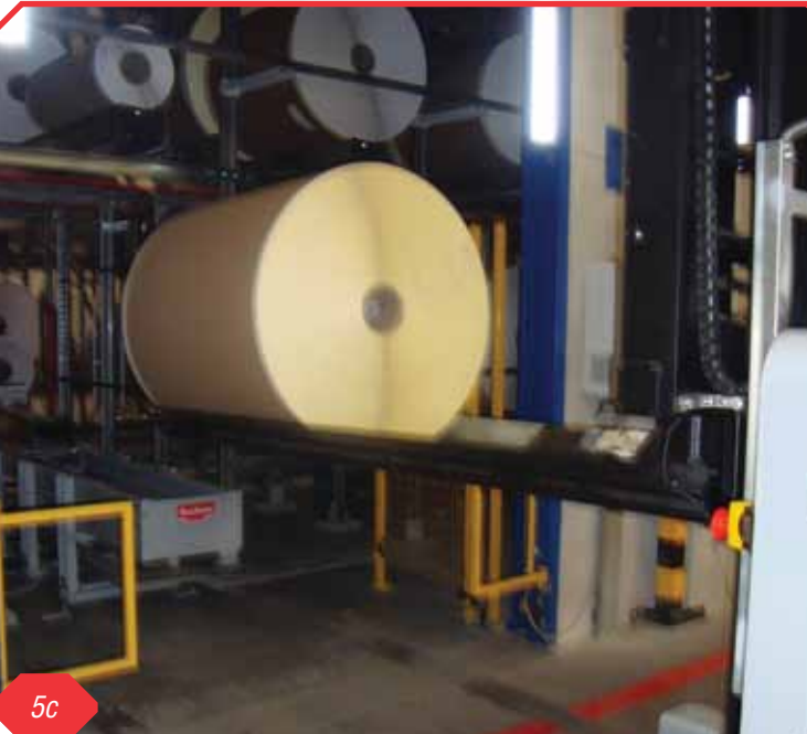
Example of integration between automatic warehouse and AGV.
