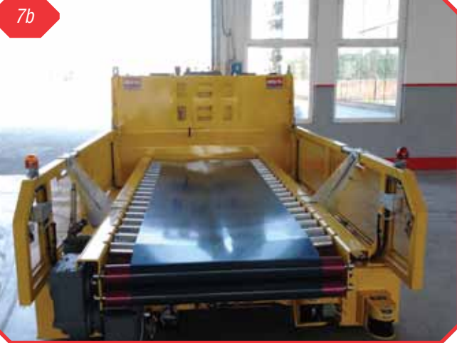
Application in paper field for mother reels. Handling solution for reels up to 10 tons
