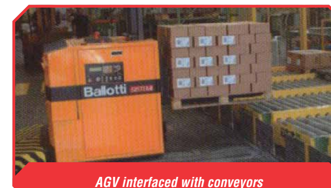
AGV interfaced with conveyors
