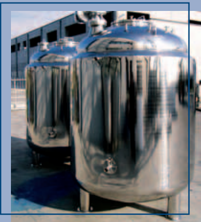
Serbatoi PED lt. 3.000 per preparazione sciroppi Vessel according PED lt. 3.000 for syrups Tank PED lt. 3.000 für die Sirup Reservoir PED lt. 3000 pour Sirops
