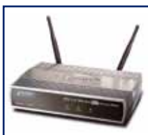
WNAP-1120PE Wireless Access Point (2T/2R) 300Mbps 11n - Porta PoE
